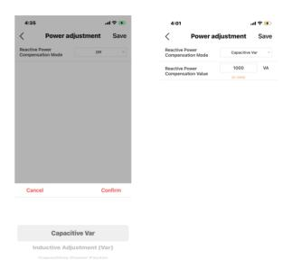
Step 1: Select Inductive Adjustment Var or Capacitive Var according to your local grid regulation. The power range is from -60%Pn 60%Pn.
