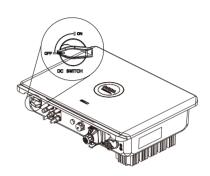
7.Connect the positive and negative connectors into positive and negative DC input terminals of the inverter, a "click" should be heard or felt when the contact cable assembly is seated correctly.
